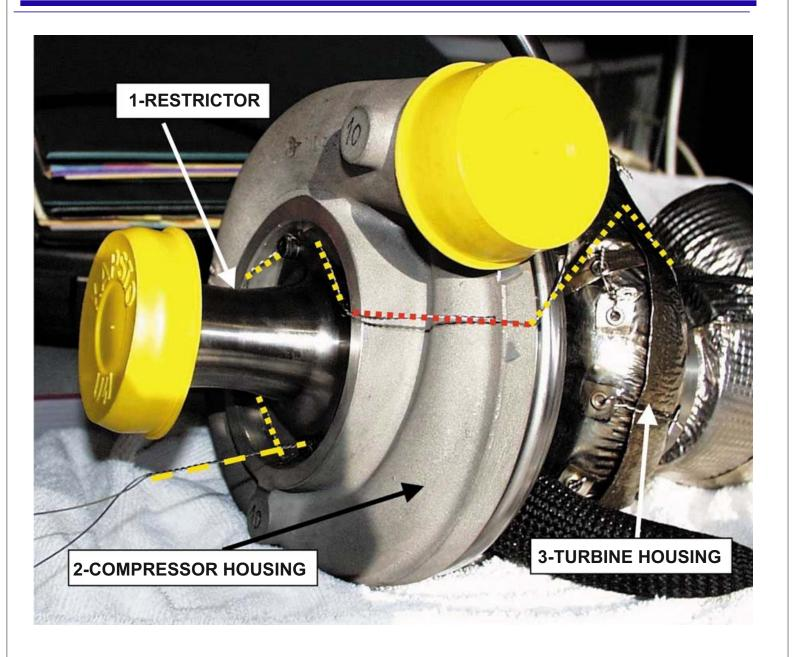
The articles 254-6.1 (Group N) and 255-5.1.8.3 (Group A) from Appendix J state: The restrict must be made from a single material and may be pierced solely for the purpose of mounting and sealing, which must be carried out between the mounting screws, between the restrictor (or the restrictor/compressor housing attachment), the compressor housing (or the housing/flange attachment) and the turbine housing (or the housing/flange attachment) (see drawing 254-4).
